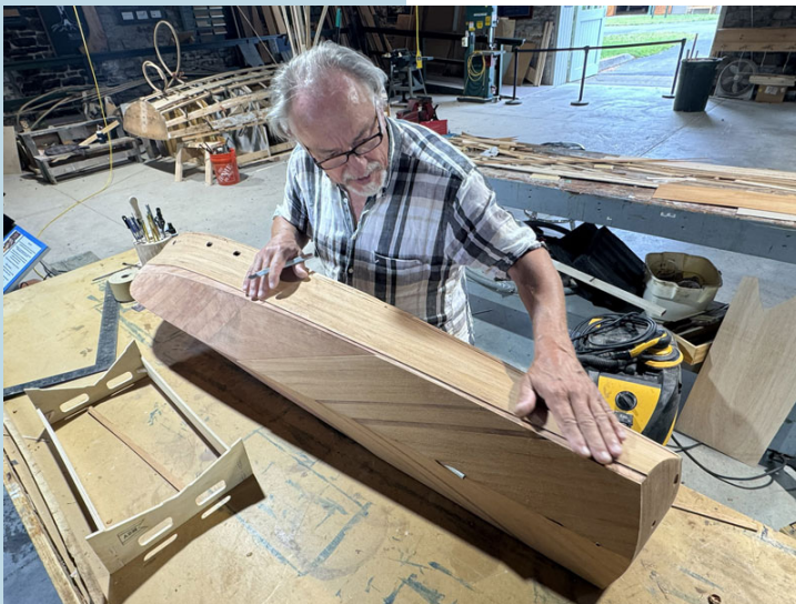
Julius adding planking to the hull.
