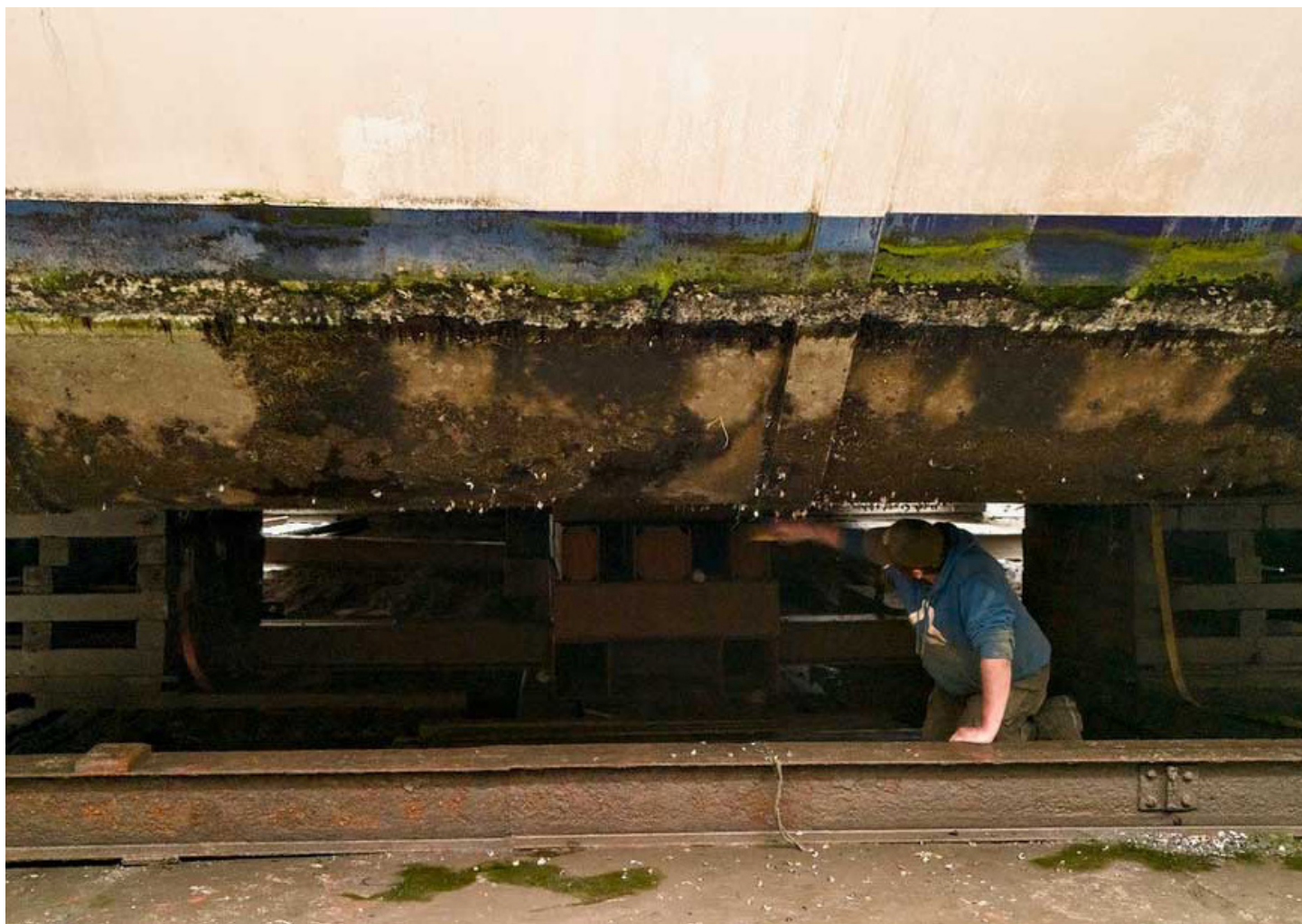
One of the Davis Dry Dock's workers cleaning La Duchesse's hull. Photo by Mike Hill, Aerosnapper.
