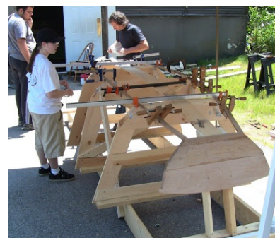
Building Daisy 12' Dory/Skiff at Turners Falls High School
